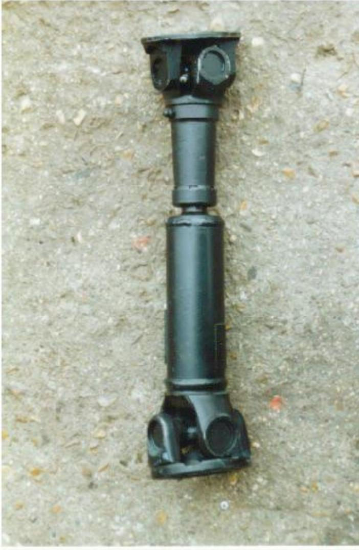
**Small bike propshaft with slide fig 7**
